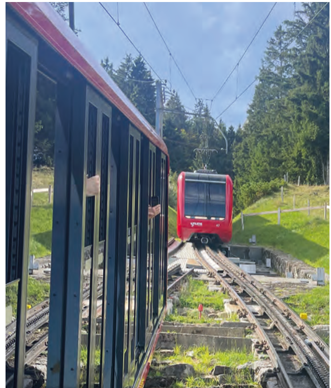
Waiting at the middle station to let the other train set cross. The train is over the sliding point plate.
