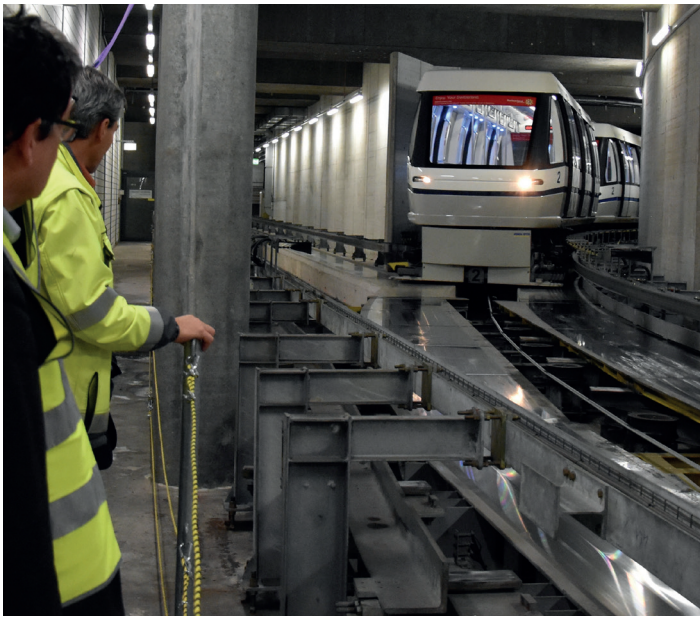
A three-car Skymetro negotiates the crossover under Zurich airport's Terminal E to reverse direction.
