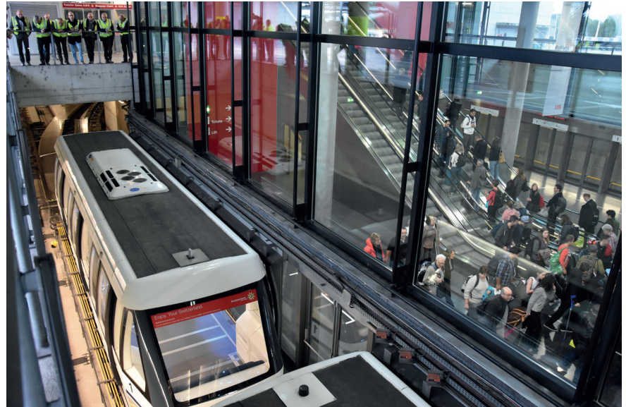
IRSE Swiss Section members overlook the Terminal E station of Zurich airport's driverless Skymetro. Just ahead is the crossover that will take the three-car train onto the other track so it can return to Terminals A and B.
