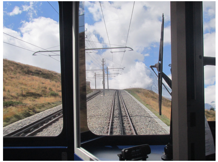
Three views of the Gornergrat Bahn, subject of the first paper. Top left, view from the cab shortly after leaving Zermatt. Above, view from the cab on the higher double track section, note the 3-phase overhead line equipment and the Matterhorn already 'in the cloud' in the centre. Left, about to depart from the Gornergrat summit station.
