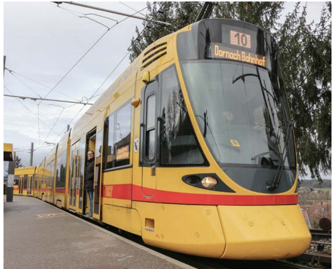
Left, innovation in regional transport. Metre-gauge electric railcar of Aare-Seeland mobil, giving full access for handicapped people using a low-floor train entrance and elevated platform. Right, innovation in urban transport. TANGO low-floor trams of Baselland Transport allowing short dwell times and increased accessibility by use of more doors and a low-floor entrance. Photos Steffen Schranil.
